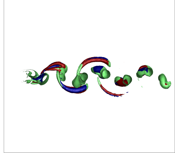
(b) Side view showing the iso-surface of the Q-criterion set to 0.25 for snapshot 65370 at Reynolds number 240.
